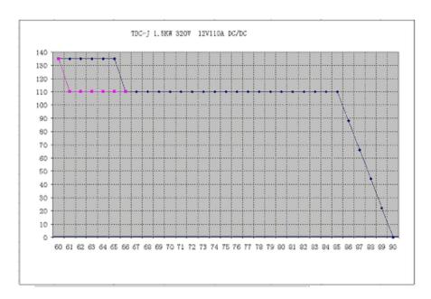
Blue line for the temperature rise of the derating curve, red line for the temperature drop of the recovery curve
